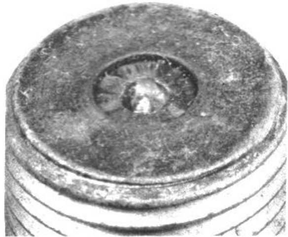
Worn-out spark plug. This amount of electrode wear can cause misfiring during acceleration or hard starting.
