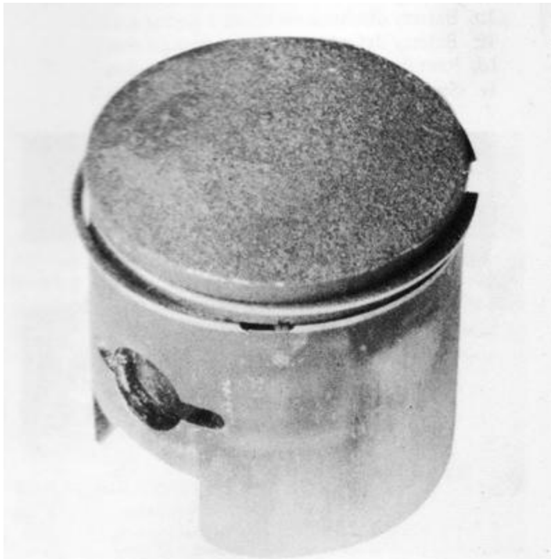
This H1 piston shows excessive blow-by past the piston rings, which have been overheated and lost tension. Note the small gap of the ring, which is an indication of lost ring tension.
