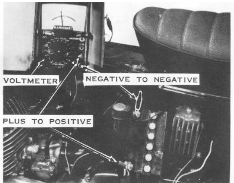
Testing the H1 battery voltage with a 30-volt DC voltmeter. It should be 12.5 volts with no load, and should not drop below 11.5 volts with the ignition and lights turned on.
