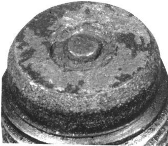
Aluminum throw-off. This is an indication of preignition. Check the engine to determine the extent of damage. Replace the plugs.
