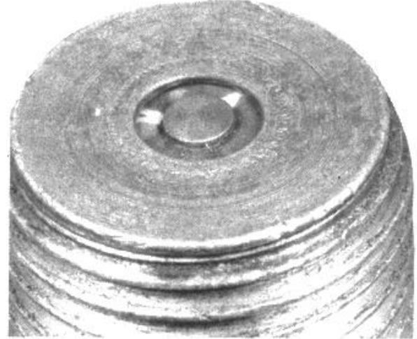
Concentrated arc. The multicolored appearance is a normal condition, caused by electrical energy consistently following the same firing path. The arc path will generally change with deposit conductivity and gap erosion. This spark plug does not need to be replaced.
