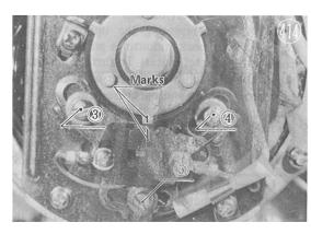
(iii) Align pointer (6) with the next mark on the rotor, and turn the rotor to check that any two points will coincide with the pickup mark and the pointer, respectively. Once the pointer is set correctly, it can be used as a reference mark to restore timing any time the pickup coil is removed or the gap adjusted.
