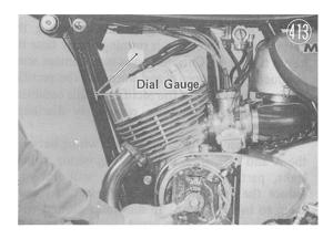
(ii) In this position, loosen the three pickup coil base plate mounting screws (3(4)(5). Align the mark on the SG magnet projection with the mark on top of the pickup coil housing, and tighten the screws back down.
