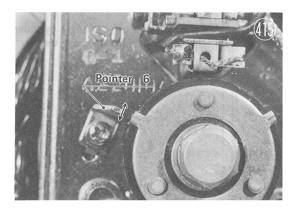
(iv) Last, ascertain that the pickup coil/magnet gap has not changed.
