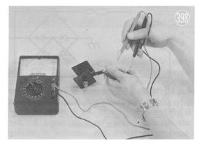
NOTE: In many ohmmeters (multi-testers) the batteries in the tester are reversed so that the negative lead is actually the positive side of the batteries inside. If this is not the case with your meter, the direction of current flow will appear to be opposite that shown in the table.
