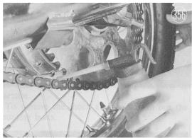
With the motorcycle in its normal standing position on the front and rear wheels, check chain play at the center of the chain as illustrated. Play must be more than 3/8" (10 mm) and should never be allowed to exceed 1 1/2" (40 mm). Adjust the chain using the chain adjusters if it is out of tolerance. Standard adjustment is 3/4" (20 mm).
