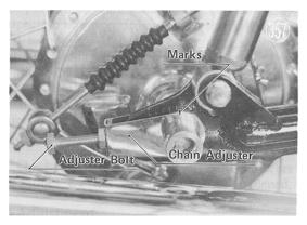
Oil the chain with SAE 90 gear oil at least every 200 miles (300 km). The H2 has a chain oil tank for this purpose, with a hose running down to drip oil on the chain. To oil the H2 chain, spin the rear wheel backward while pulling up on the oiler valve knob (attached to the frame at the rear of the engine oil tank).
