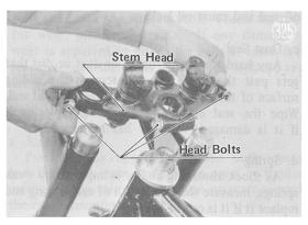
Remove the steering stem bolts and pull out the front forks and covers.
