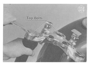
Take out the steering stem head bolts and remove the stem head. (Disc brake models)
