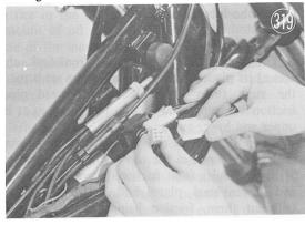
Take off the speedometer and tachometer cables and remove the meters, bracket and ignition switch as an assembly.
