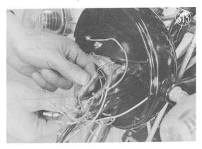
Remove the starter, throttle, clutch and front brake cables from the handlebar. On disc brake models, remove the complete disc brake assembly in one piece.
