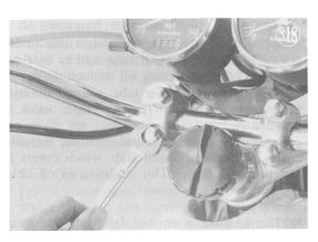
On disc brake models, remove the fuel tank and undo the ignition switch and left handlebar switch wiring.
