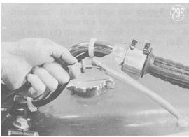
Loosen the front brake adjusting nut and pull the cable off the brake lever. (Expansion brake models)
