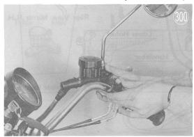
Loosen the handlebar mountings, remove the right upper mount, move the handlebar to the left for easy cable removal, and tighten the left mounting.
