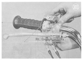
Pull the throttle grip off together with the bottom
