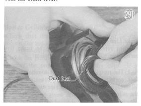
Remove the oil seal from the cylinder.
