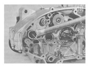
Turn the crankcase assembly upside down and remove the mounting nuts.
