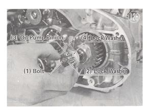
Straighten out the lock washer.
