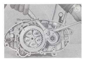
Remove the lock washer, distributor pinion and primary gear. (H1)
