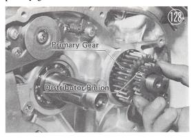
Remove the lock washer and primary gear.
