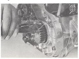
Temporarily mount the clutch housing and clutch hub, and holding the crankshaft stationary with a clutch hub mounting tool (special tool), remove the nut.
