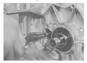
NOTE: Removal of the oil seal or push rod bushing necessitates disassembly of the crankcase.
