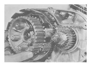
Last, pull off the bushing and the other thrust washer.
