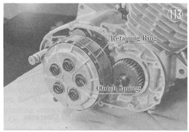
Remove the spring guides, spring plate, steel plates, friction plates and steel rings.
