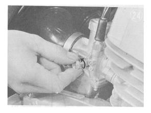
With all the throttle valves fully closed, adjust the outer sleeve of each throttle cable for zero play. Accomplish this by turning throttle cable adjuster C right or left, while moving the cable sleeve up and down until no play is felt. Don't fail to tighten lock nut D after adjustment is made.
