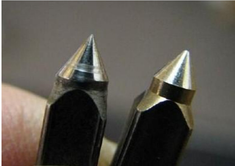
Worn float needle vs. new kit needle
